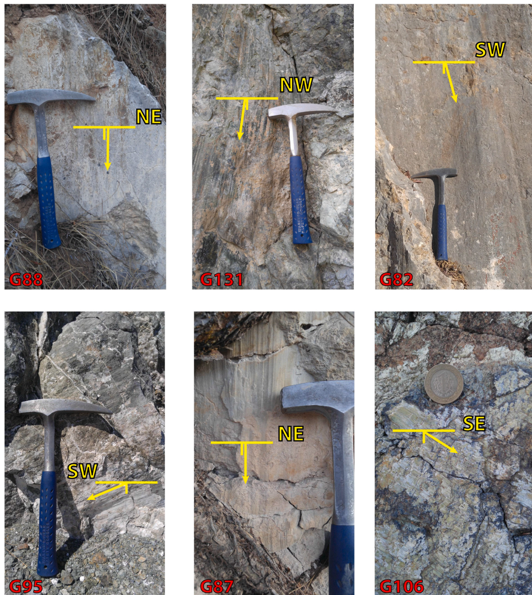
Fig. 5. Slickensides on various fault planes. Arrows indicate the sense of slip of the hanging-wall block. Note that G95 is a NE-SW striking fault with dextral component and G106 is a NW-SE striking fault with a sinistral component. All others are normal faults.
